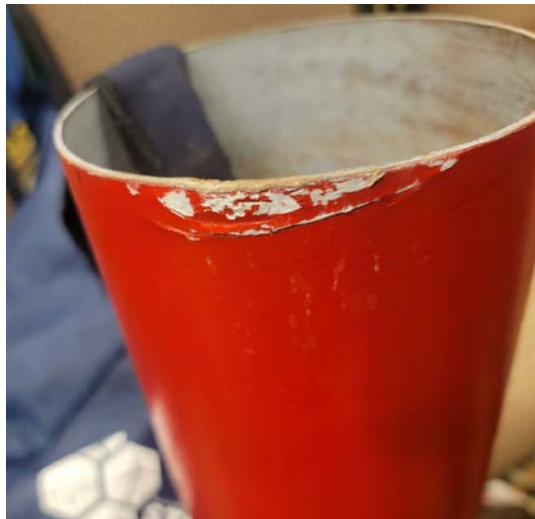
This picture displays the damage done to the upper bottom section to the rocket. This damage corroborates the theory that the rocket had a rough landing on a hard surface.
