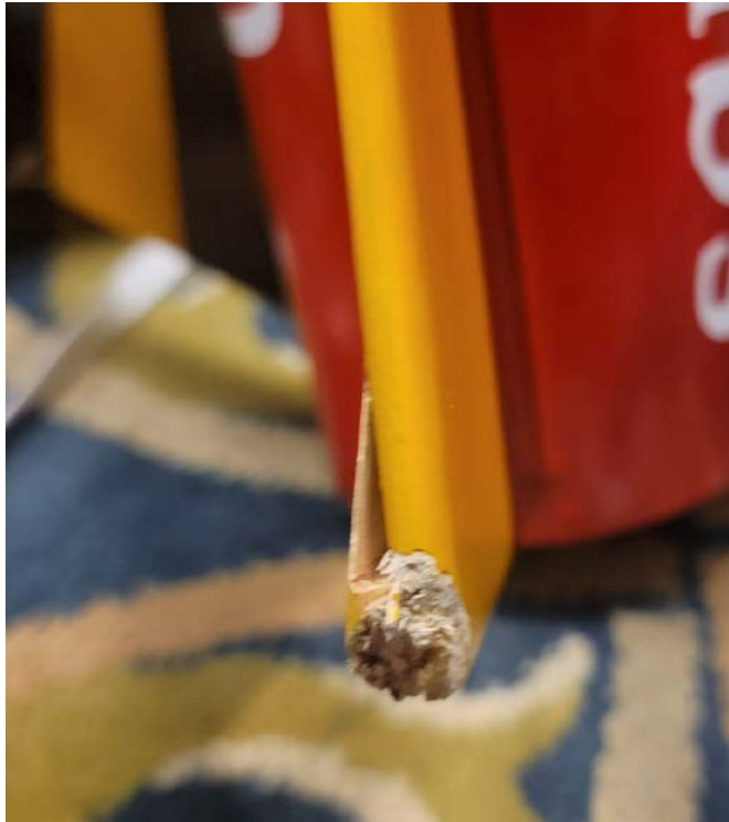
After we evaluated our rocket for damage, we spotted this. The fin must have been hit and the plywood split. This would take a bit of work to fix, but it is repairable.
