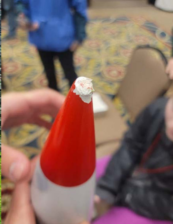
The damage to the nose cone can be seen here. Most of this is just paint damage but a bit of the plastic also got crushed when landing.
