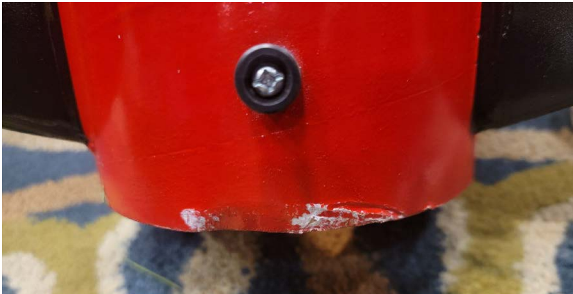
Here is the post-launch damage to the outer bottom tube of the rocket. This damage tells us the rocket had a rough landing and must have hit a hard surface.
