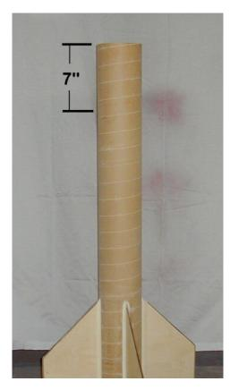
9.2 Mark a spot 7 inches down from the forward end of the booster tube. Drill a 3/16" hole at this point.
