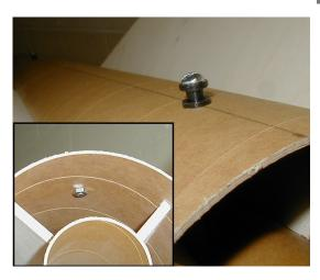
5.5 Screw the rail buttons into the two holes using the #8 - 1/2" screws. Install the #8 nut on the screw to secure it.
