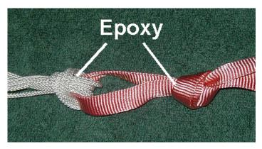
**8.4** Put a small amount of epoxy on the knots to ensure they do not unravel.
