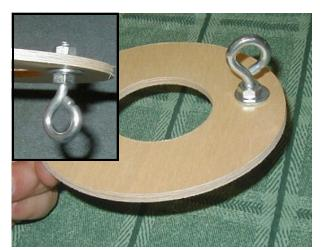
2.2 Mount an eyebolt through the 3/8" hole in the Forward Centering Ring. Install a nut / washer on the top side of the centering ring and a washer / nut on the bottom. Tighten the nuts and secure both nuts with a drop of epoxy.
