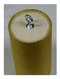
**7.2** Recess the bulkhead 1/8" into the 11" long payload coupler. Epoxy the back side of bulkhead in place using stick or similar item. Once cured, epoxy the front side using a straw or similar item.
