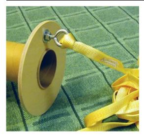
3.1 Attach the 40 ft. shock cord to the Forward Centering Ring by passing the loop at one end of the shock cord through the eye-bolt in the Front Centering Ring. Now pass the rest of the shock cord through the loop and pull snug. Place a little epoxy on the knot to secure it.
