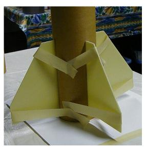
**4.5** Use masking tape to hold the fin in position while the epoxy cures. Repeat this process for all fins. Allow the epoxy to fully cure before proceeding to the next step.
