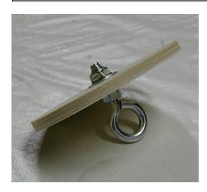
7.1 Mount an eyebolt through the 3/8" hole in the bulkhead. Install a nut / washer on the top side of the shock cord mounting ring and a washer / nut on the bottom. Secure both nuts with a drop of epoxy.
