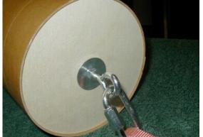
8.2 Attach the shorter end of the Tubular Nylon Cord to the eyebolt in the payload section using the quick link as shown
