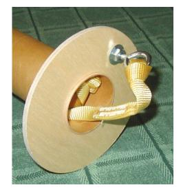
3.2 Now place the shock cord into the motor tube to keep it out of the way for the next step.
