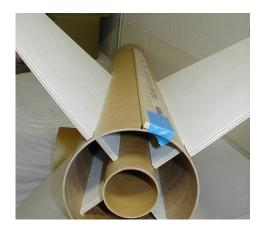
5.3 Using a straight edge (a yard stick works well) site down the body tube and draw a line parallel to the center axis of the tube.
