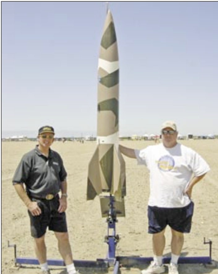
Karl Baumann and Andy Woerner stand next to Andy's 10" diameter V2 flown with the first 98mm M750W long burn motor at the Dairy Aire 2007 launch near Fresno, CA (photo by Gary Rosenfield).
