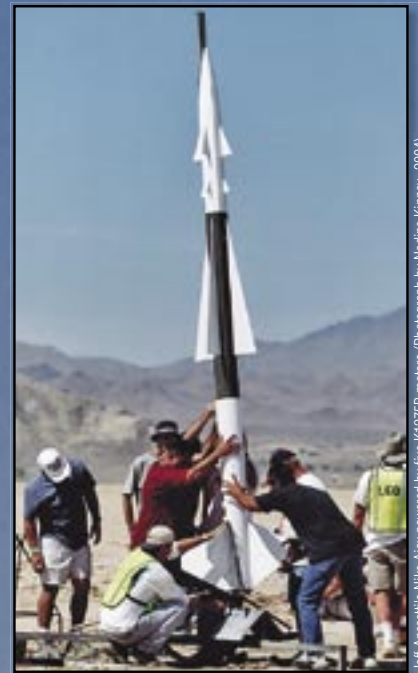
Jeff Aneseth's Nike Ajax powered by five K1276R motors (Photograph by Nadine Kinney-2004).
