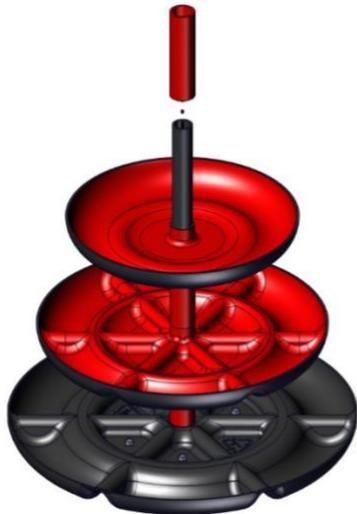
11. Press the same color Pipe Cap (am-4297\_Red or Blue) onto the end of the inner pipe.
