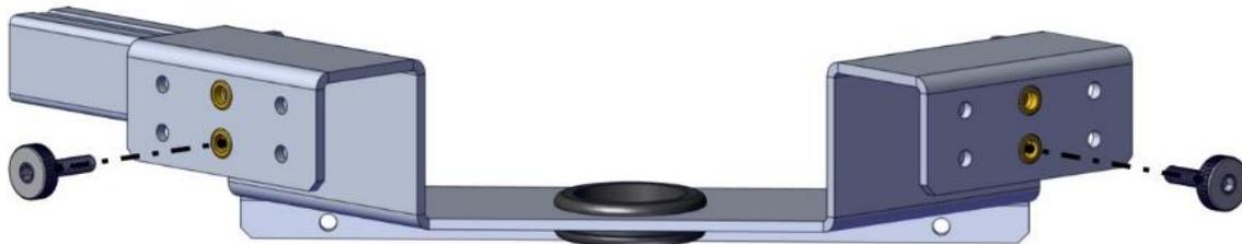
12. Insert a Grommet into the center hole in the Bottom Carousel Support Bracket.
