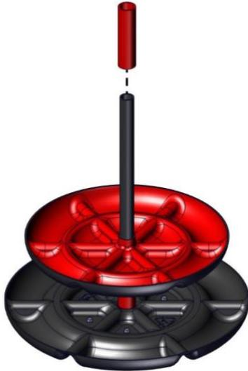
9. Add the same color Upper Tray (am-4493\_Red or Blue) to the assembly by pressing the center of the tray onto the pipe. This is Level 3.
