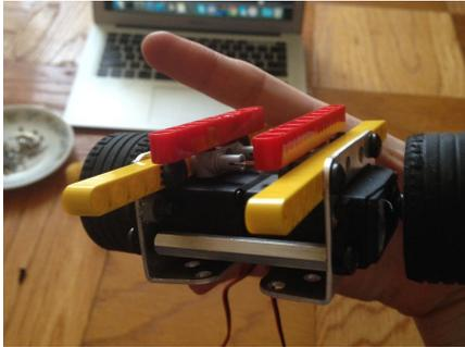
The picture here is the drivetrain of the Scorpio robot. Scorpio utilizes a wheel-motor drivetrain, with its wheels mounted via the classic servo horn method. Instead of using the standard chassis to connect our drivetrain, our team decided to use a very tight, two-servo-horn-and-standoff method. This gave us numerous benefits such as having a smaller turn radius and freeing another robot to use the chassis provided in the parts list.
