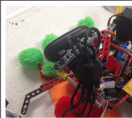
We sandwiched the two flaps of the camera between two lego beams, which were connected by standoffs in order to prevent shaking. Another proposed idea was to put lego beams around the head of the camera itself. We ended up not going in this direction as it was a less secure mount that added an additional layer of inconsistency we felt was unnecessary.
