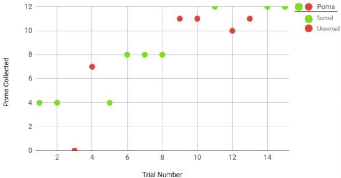
This graph shows how many poms Scorpio was able to collect for each run as well as whether or not the poms collected were color sorted. For each trial, Scorpio would run its path and attempt to obtain a maximum of 12 poms. We would record how many of the 12 poms Scorpio would collect and add a data point to our graph. If Scorpio's red
