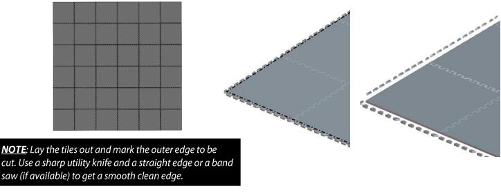
**Step 1-3 Optional:** Locate the following locations on the floor. In order to get the Balancing stone to fit, the corners of the tiles may need to be trimmed.
