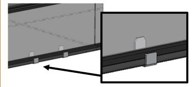
**Step 3-3:** Locate two Beam Clamp Assemblies and loosen the screws enough to fit over the field perimeter.
