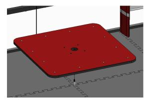
**<u>Step 4-7</u>**: Secure each Balancing Stone to the protruding bolt with a 1/4" washer and 1/4"-20 nut. Tighten the nut until it hits the standoff.
