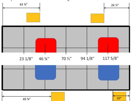
For AndyMark, IFI and LogoLoc perimeters, targets can be hung in place with Command Adhesive Mini Hooks. For early generation AndyMark Perimeters, use Velcro Dots to hang the targets.
