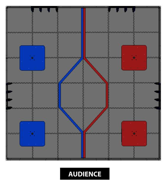
RED and BLUE tape should be placed one either side of the field center line and starting from the perimeter wall furthest from the audience and extending the length of two tiles. The tape should form 45 degree angles to form an elongated hexagon shape.
