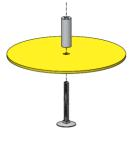
**<u>Step 4-4</u>**: At the intersection of four tiles, slide the disk portion of the assembly underneath.
