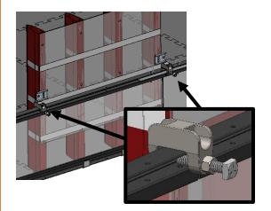
**Step 3-5:** Tightly secure the Cryptobox to the Beam Clamp using a cable tie.
