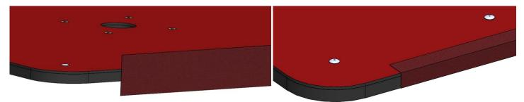
**Step 4-2:** For the Corners, start with a strip of tape, then cut the top portion into roughly half inch tabs. This helps to make the top surface smooth for robots driving on the top surface. Fold each tab over onto the top surface of the Balancing Stone. Fold the bottom portion under the main plate, be sure to flatten any large wrinkles. There should be no gaps between the edge tape and the corner tape.
