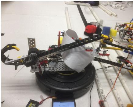
On our create we have a claw attached to an igus chain, allowing it to change elevation and reach the pomps on the terrace. Initially, we considered using a standard claw on a rod attached to a fulcrum. We ended up not going with this design as when the claw was raised it stopped being parallel to the ground unlike with the igus chain.
