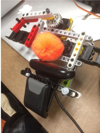
We sandwiched the base flap of the camera between two lego beams which were connected by axles to secure it. We alternatively considered putting lego beams around the head of the camera itself. We ended up not going with this strategy as it was looser than the alternative, meaning that the poms would have always been in different locations in the camera's view.
