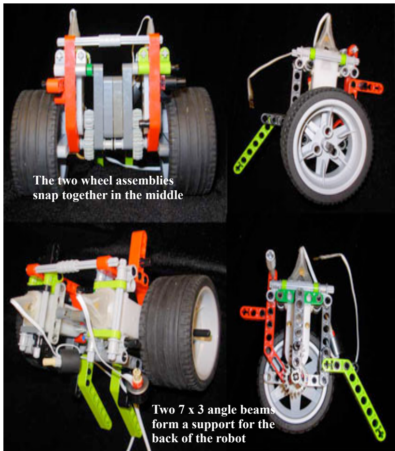
Figure 3 Prototypes: Wheel Assembly and Gear Train
